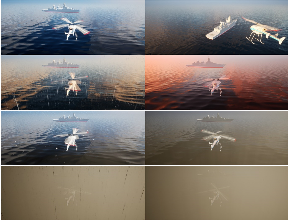
Figure 3, a-h: Simulation of different ODD parameters utilizing the SenSim2 framework, showcasing effects of rain, snow, fog, and daylight.
